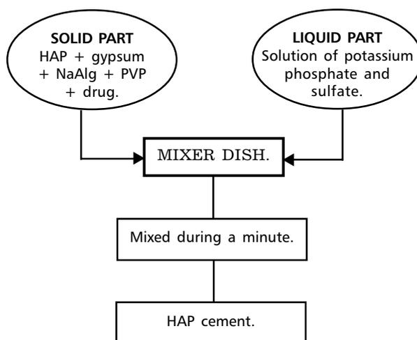
Fig. 1. Preparation scheme of HAP + gypsum + polymers cements.
